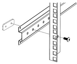
a. Unscrew the rail from the rail support. Move the rail forwards or backwards to desired location. Insert screw and secure.
