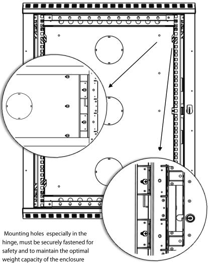
a. Finish installing the enclosure by securing screws along the inner mounting pattern and through the hinges.
