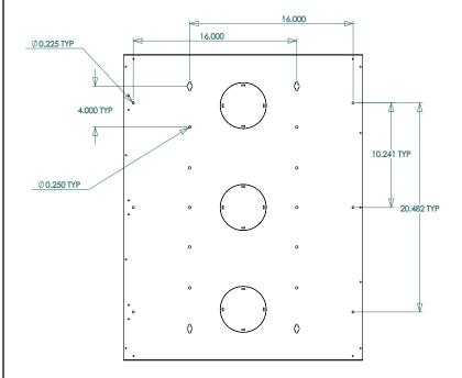
a. Using the dimensional drawing above, mark the desired placement of the mounting holes on the wall.
