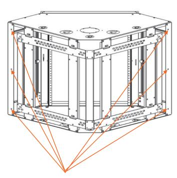
Install screws (not provided) in these six (6) locations <u>BEFORE</u> installing any equipment in the cabinet. \*Warranty Disclaimer \*
