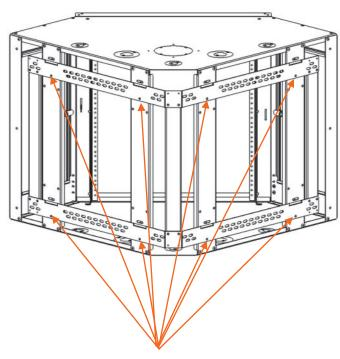
(Optional) Install wallmounting screws (not provided) for additional security in these eight (8) locations to secure the cabinet to the mounting frame.
