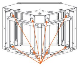
Once mounting frame is secured to corner, lift and lower the wallmount cabinet so that each of the eight (8) beveled tabs slides into the eight (8) slots in the back of the wallmount cabinet.
