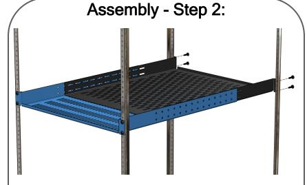
Place the Extension Shelf inside the Base Shelf with the mounting ears adjacent to the back rails and attach using the correct fastener for your type of rack rails.
