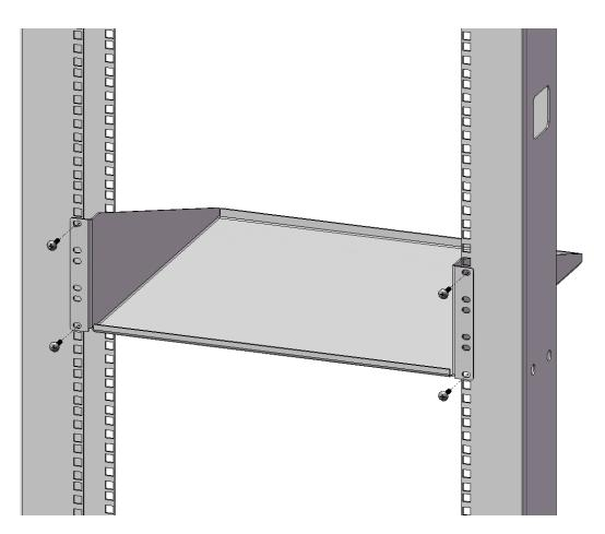
The Kendall Howard 3U Component shelf will mount to any 19 inch EIA-310D compliant racking system. Attach shelf to rack rails with mounting hardware as shown above. (Hardware used is specific to your rack rail system but should be 10-32, 12-24, M5 or M6 hardware)
