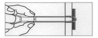
4. Place your thumb between the plastic straps and snap the straps off.
