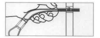
3. Pull the wing firmly against the inside wall of the hollow material using the ring, then slide the plastic cap forward until the flange is seated flush against the work surface.
