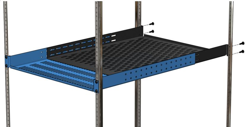
Place the Extension Shelf inside the Base Shelf with the mounting ears adjacent to the back rails and attach using the correct fastener for your type of rack rails.
