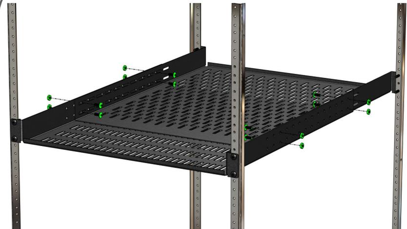
Bolt shelves together through the closest aligning slot and round hole to each rail with hardware provided. The further apart the bolts are from each other, the stronger the shelf will be.
