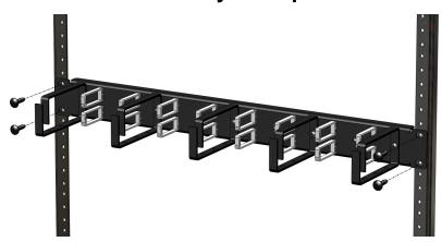
Use cage nuts (if needed) and rack screws to fasten Cable Management Kit to rails, secure with screw driver.
